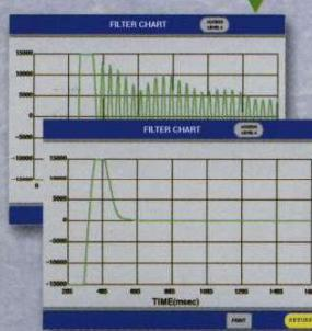
Digital filtering of the load cell signal
